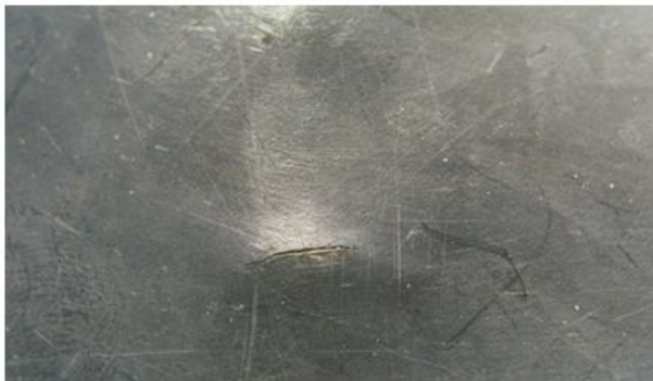
Early stage of stress puncture by angular-semi-rounded stone
